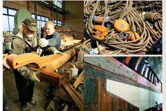
Sealing the oak planks with traditional methods, oiled hemp oakum hammered in with a chisel
